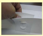
6 Remove backing tape, insert both semicircle tabs through the horizontal slits to secure the panels in place. Prefold the semicircle tabs to allow easy insertion. of the tabs.
