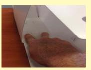
7 Secure the tabs in place from inside the box. Firmly press down at the same time to adhere the tape in position.
